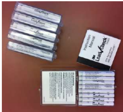
Lead Check Swabs: 'red means lead'
